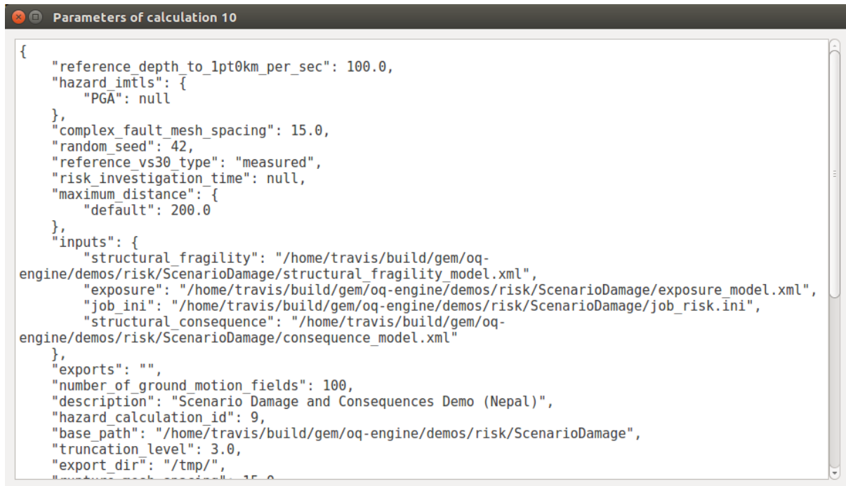
Fig. 15.3: Example showing parameters of a OQ-Engine calculation
