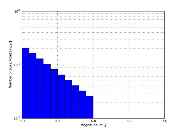
Fig. 2.6: Example of a double truncated Gutenberg-Richter magnitude-frequency distribution.
