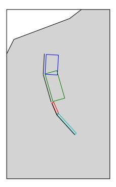
Fig. 2.4: Geometry of a multi-segmented characteristic fault composed of four rectangular ruptures as modelled in OpenQuake.
