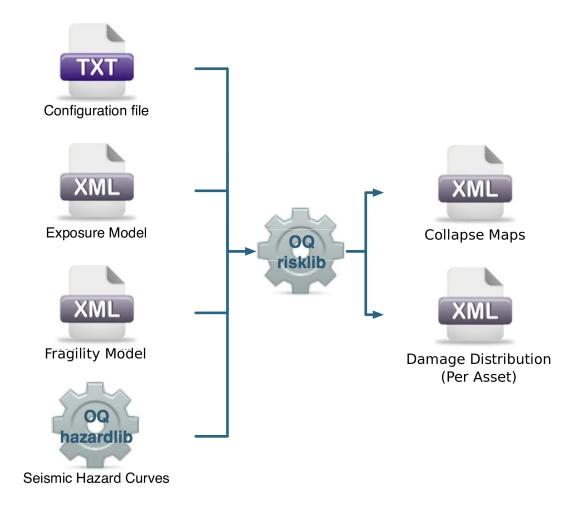
Fig. 3.3: Classical PSHA-based Damage Calculator input/output structure.
