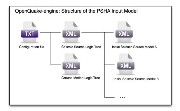
Fig. 2.9: PSHA Input Model structure
