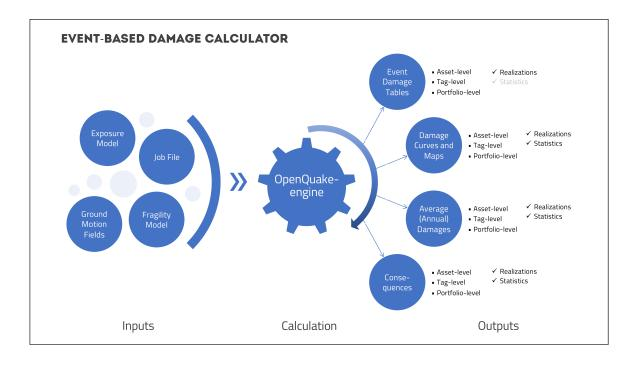
Fig. 3.5: Probabilistic Event-based Damage Calculator input/output structure.
