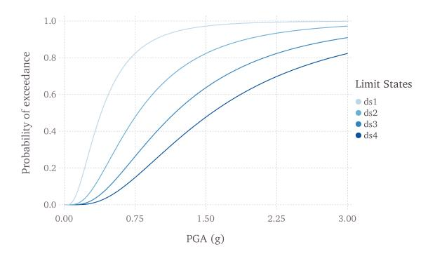
Fig. 3.14: Graphical representation of a continuous fragility model
