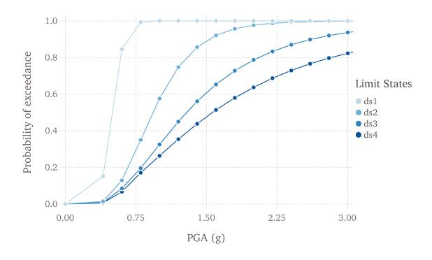
Fig. 3.13: Graphical representation of a discrete fragility model
