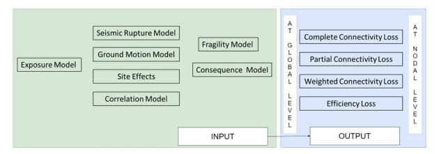
Fig. 3.11: Input models required, and output obtained in OpenQuake for infrastructure risk assessment at connectivity level
