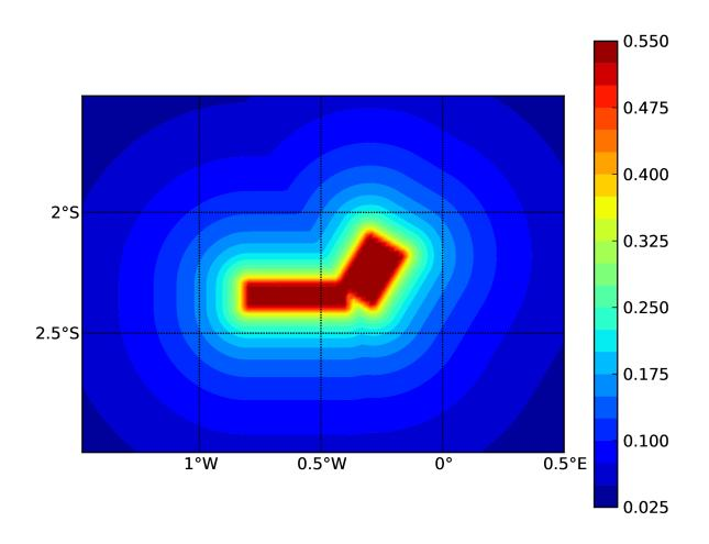
Fig. 2.17: characteristic fault source with collection of planar surfaces
