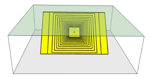
Fig. 2.2: Point source with multiple ruptures. Note the change in the aspect ratio once the rupture width fills the entire seismogenic layer.
