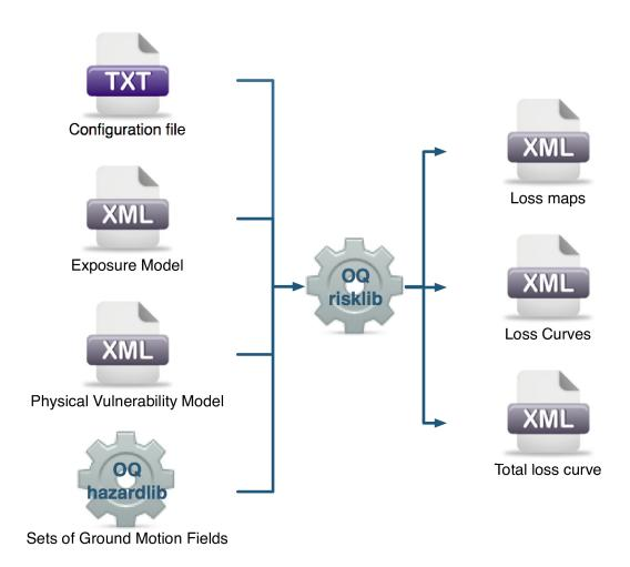
Fig. 3.6: Probabilistic Event-based Risk Calculator input/output structure.
