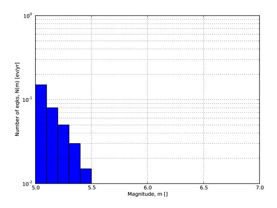
Fig. 2.5: Example of an incremental magnitude-frequency distribution.
