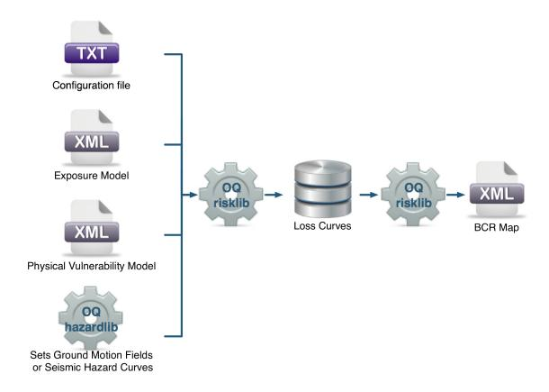
Fig. 3.7: Retrofitting Benefit/Cost Ratio Calculator input/output structure.
