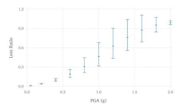
Fig. 3.16: Graphical representation of a vulnerability function that models the uncertainty in the loss ratio using a lognormal distribution. The mean loss ratios and coefficients of variation are illustrated for a set of intensity levels.
