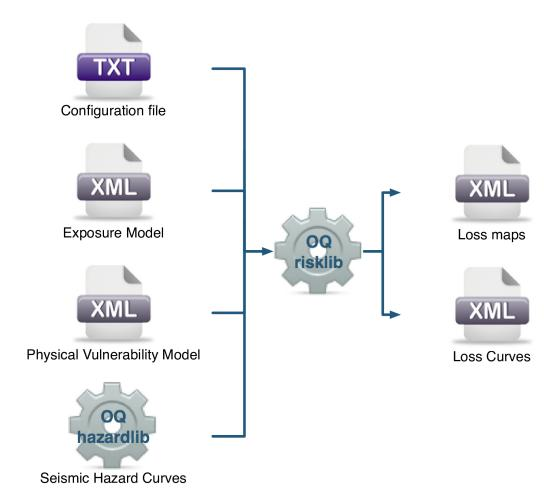
Fig. 3.4: Classical PSHA-based Risk Calculator input/output structure.
