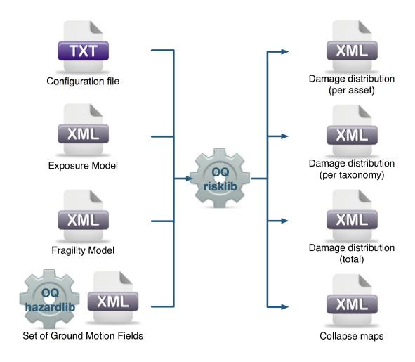
Fig. 3.1: Scenario Damage Calculator input/output structure.
